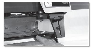
(To account for stone wear, loosen wing knob (part 64) and adjust side guard (part 60) and finger assembly back towards the grinding disc until clearance between the disc and finger is minimal.)
